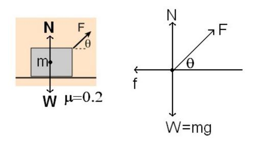
A box of mass m=20 kg is pulled by a force of F=100 N at an angle $\theta$ =53° with the horizontal.
