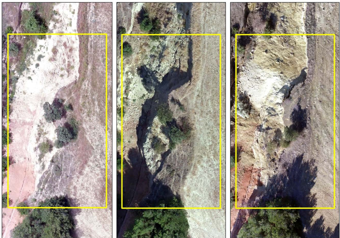
Figure 10. Landslide Progression, Left – Campaign 1, Middle –Campaign 2, Right – Campaign 3
