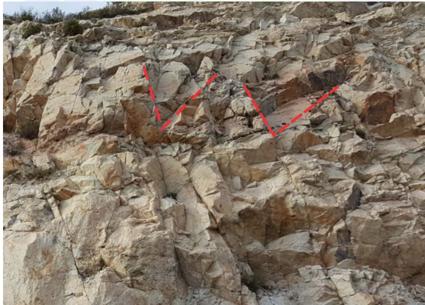
Figure 4. Potential wedge failures observed in the field.
