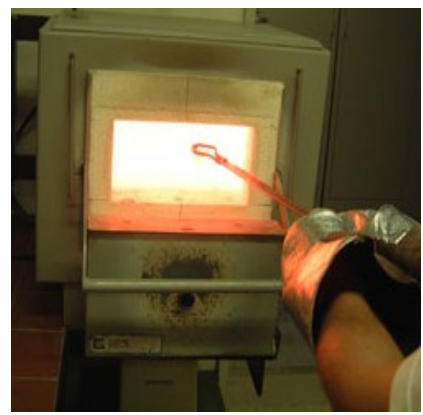
Ignite in muffle furnace 550 °C for 15-20 minutes
