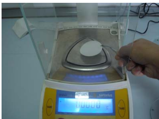
Weigh 0,45 µm membran filter
