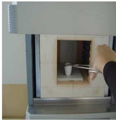
Ignite in muffle furnace 550 °C for 15-20 minutes
